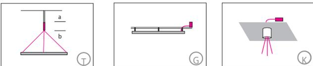
**T** Suspension with pendant canopy PB 375 and current-carrying steel cables (a) 5000 mm / 196.8" + (b) 3000 mm / 118.1"
