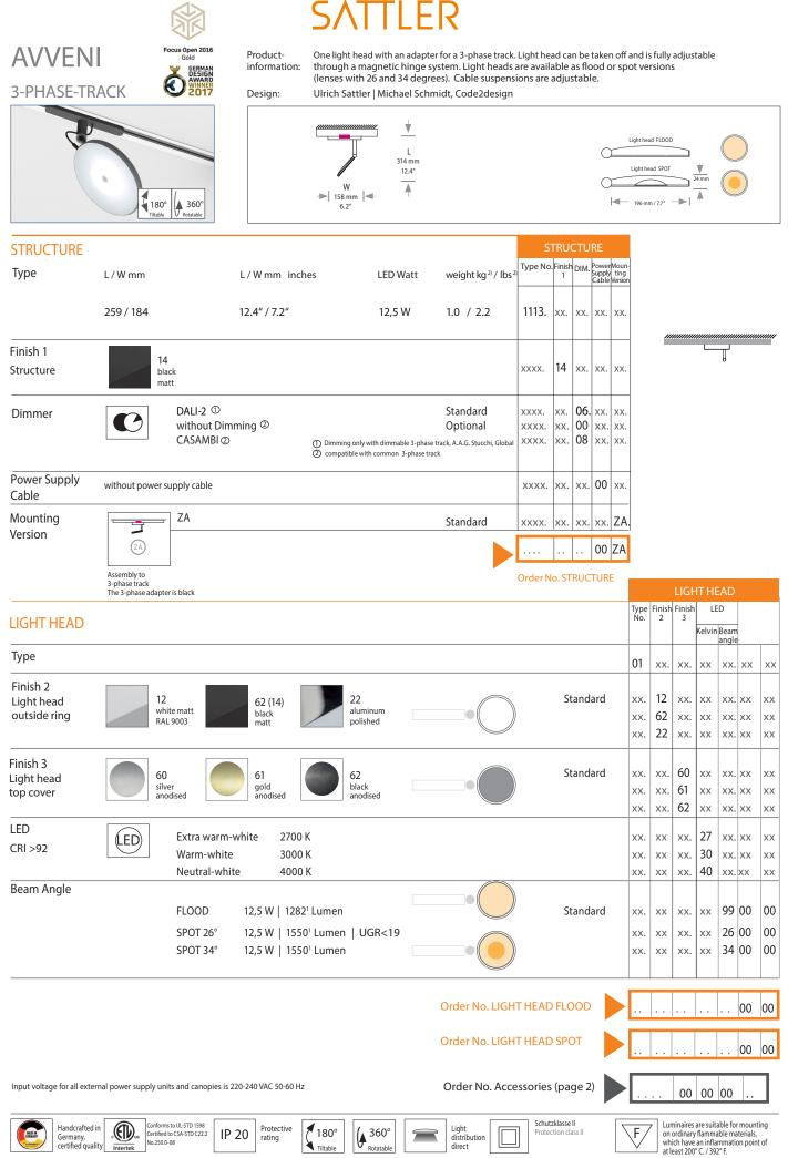
Germany, certified quality Technical data is subject to change. Errors and omissions excepted 1) Net lumen output: Losses due to diffusors and reflectors are considered. Lumen values refer to an ambient temperature of max. 35° C / 95° F. 2) Weight of lights without remote technical unit or canopy.
